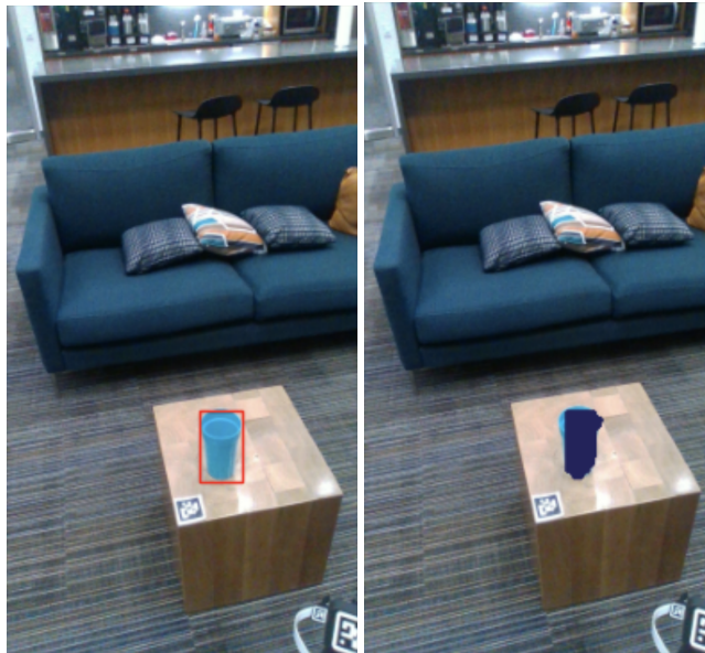
Figure 7: The robot detects and localizes the cup using YOLO-World and segments the result with FastSAM on a frame captured from its head camera for perception.
